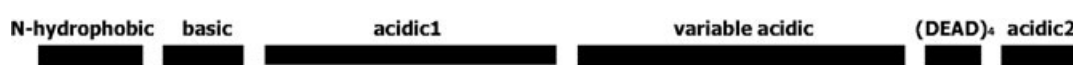
Figure 5. Schematic diagram showing the six domains present in the Asprich family of proteins: N-hydrophobic (19 residues), basic (9 residues), acidic1 (consensus sequence of 97 residues), variable acidic, DEAD domain (consensus 20 residues), acidic2 (consensus 25 residues) -C. The exact boundaries between these domains are shown by arrowheads in Figure 3.
